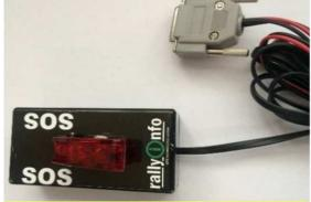
between the two seats on the floor or on the top of the cabin inside. In case SOS is needed (help is needed) only the switch under the red cover must be used (click it to other position) and the device starts sending SOS to HQs. SOS can be stopped by closing the red cover.
